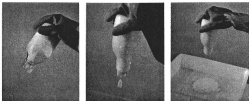
Figure 1: Slurry that is formed when a tertiary amine is used as an acid scavenger
