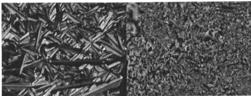
Figure 4. Left: Batonnets forming in a fan-like texture in 1P10Cl at 40 °C upon cooling (solid phase). Right: Spherulite texture of 1P10Cl·H 2 O at room temperature (smectic phase).
